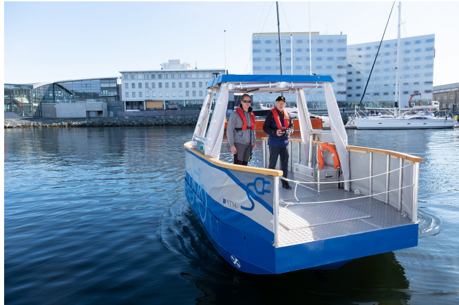
Figure 1.1: Autonomous pilot ferry Milliamper in 1:2 scaled model of the autonomous ferry that will be built in the Autoferry project. Courtesy of Kai Dragland.
