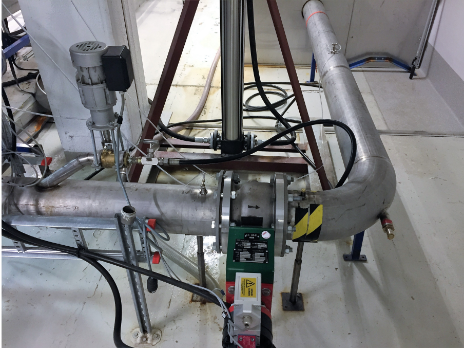
Figure 21: Compressor discharge valve at the NTNU wet gas compression test rig.
