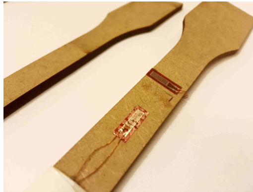
Figure 8: The two perpendicular strain gauges.
