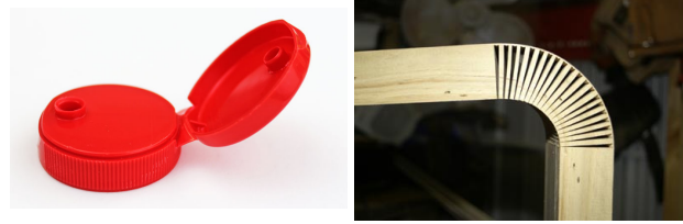
(a) A flexure from a food container made from plastic. Often referred to as a living hinge. (b) Kerf bend is a kind of flexure usually made with subtractive manufacturing in wood.
