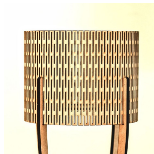
Figure 22: A lamp screen made out of MDF with an integrated LET pattern. Picture: [3]
