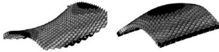
Figure 5: l. Anticlastic/positive Poisson ratio, r. Synclastic/negative Poisson ratio
