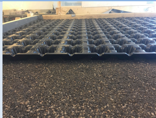
R9: Leca concrete pavers with grout material as filler, geotextile, lifted 1,5 cm
