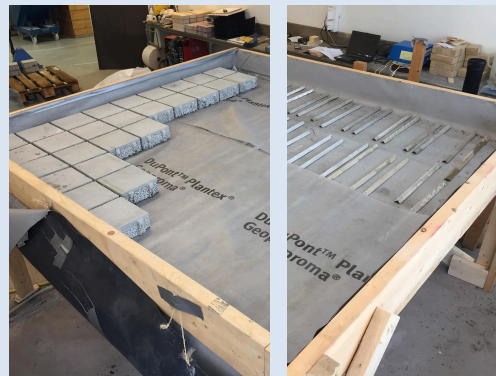
R9: Leca concrete pavers with grout material as filler, geotextile, lifted 1,5 cm
