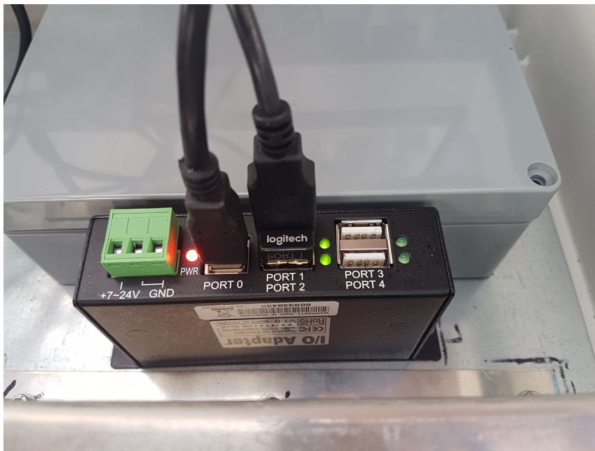
Figure 4.1: VHF transmitter connected to PORT 1 on the on-board computer
