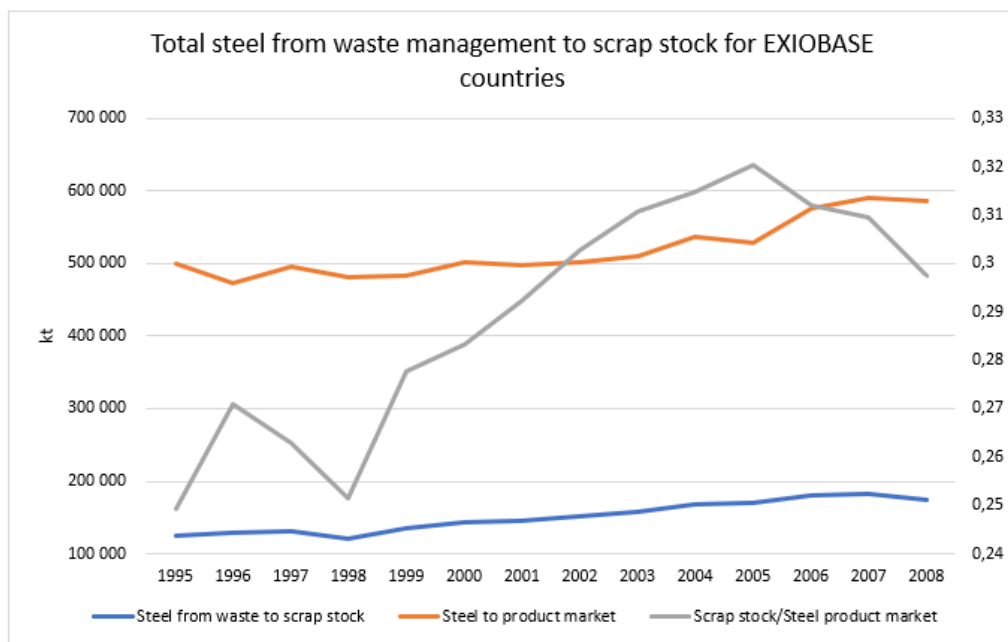
Figure 4.3: Graph of the trend of production and recycling in kilo tonnes from waste management to the scrap stock from 1995-2008 on primary vertical axis, and the ratio of recycling per production on secondary vertical axis (Pauliuk & Hasan 2017).
