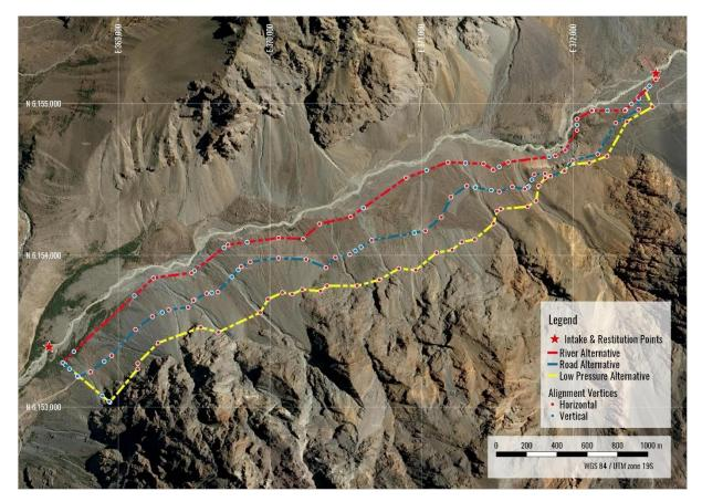
Figure 5.28: Conduits Alternatives: Horizontal Alignment
