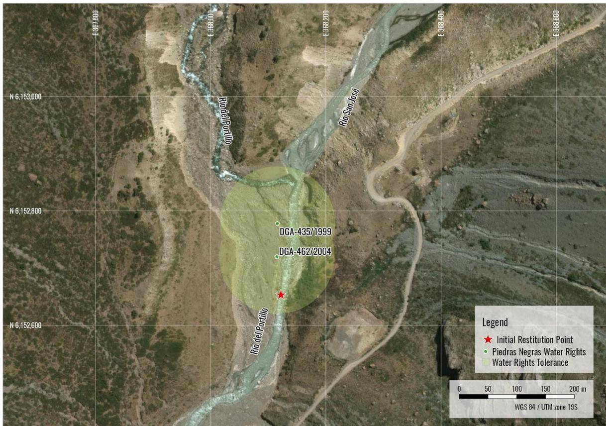
Looking at Figure 5.1, especially focusing in the green *error threshold* area, it was decided that this sector was not suitable for locating the powerhouse since it potentially exposed this structure to the flood flows from Portillo river, whose alignment at the confluence points directly to the left bank of the San José river, where the powerhouse should be located.
