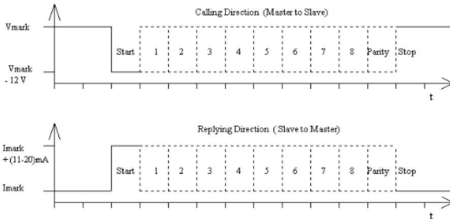
Figure 3.3: Transmission of a single packet in M-Bus
