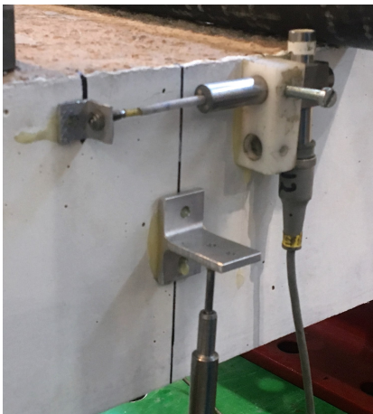
(a) LVDTs in the front of the beam
