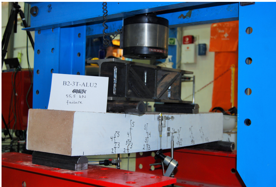
Figure 6.12: Crack development of beam B2-3T-ALU2
