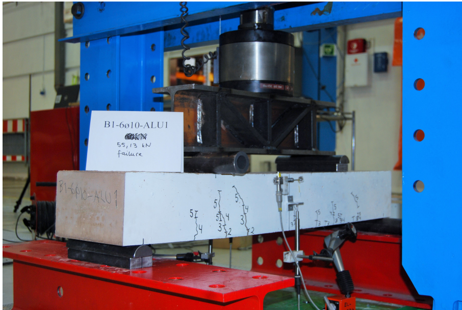
Figure 6.16: Crack development of beam B1-6ø10-ALU1
