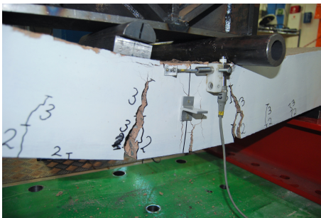
(a) Closer look on the large bending cracks
