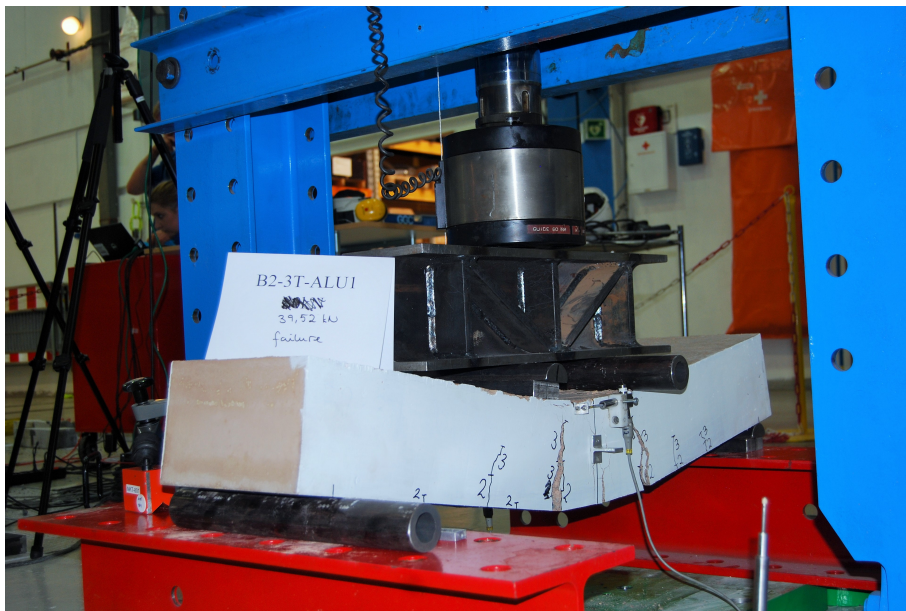
Figure 6.8: Crack development of beam B2-3T-ALU1
