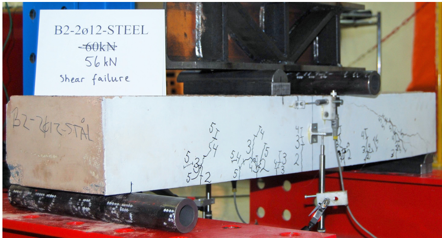
Figure 6.3: Crack development of beam B2-2 \phi 12-STEEL
