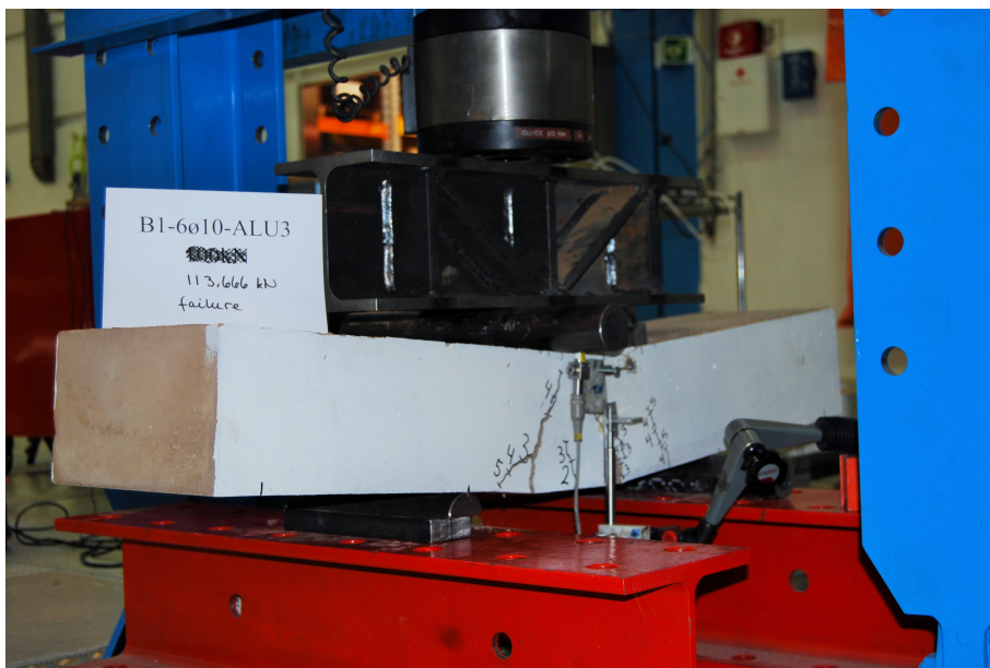
Figure 6.22: Crack development of beam B1-6ø10-ALU3
