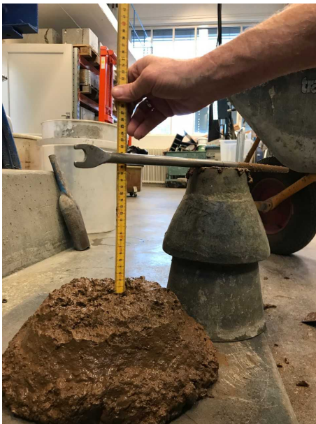
(a) Slump test
