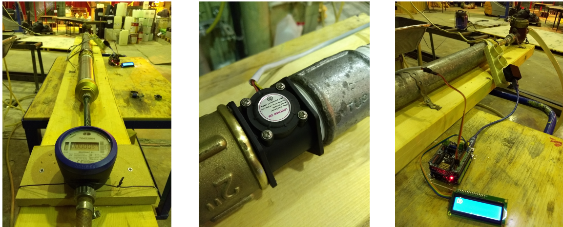
Figure 4-2: 1: The horizontal pipe fitted with a conventional water meter. 2: The NCA sensor. 3: The module for storing and transferring data & screen for displaying the water flow.
