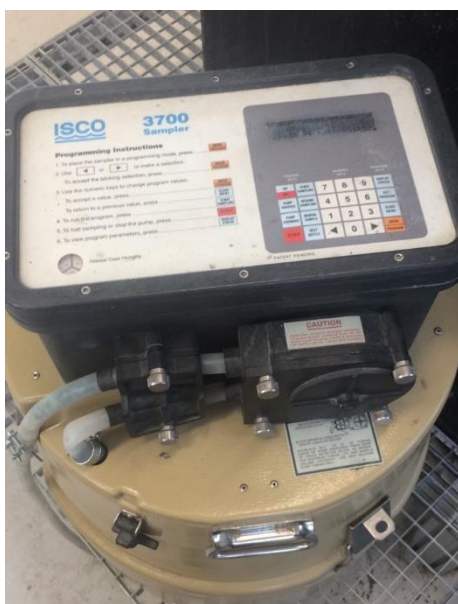
Figure 31 The automatic composite sampler for effluent samples placed by the outlet of the reactor
