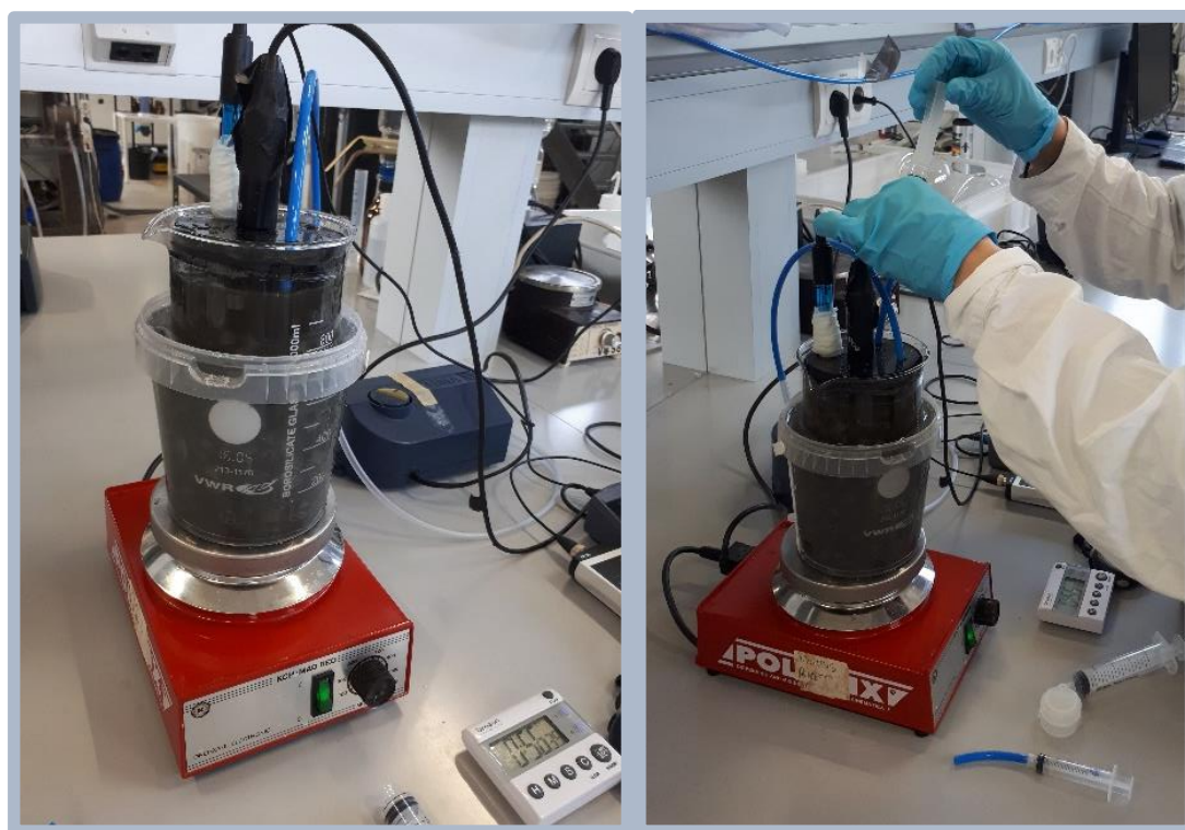
Figure 35 - Set-up of Kinetic Experiments. When no control of temperature was needed the container loaded with ice, in which the beaker was placed in, was removed
