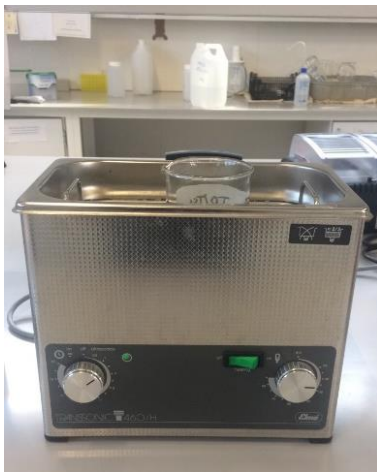
Figure 33 - Elma Transsonic T 460/H Ultrasonic Cleaner used for detaching biomass on carriers so that the TP content on the biomass could be established.
