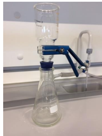
Figure 34 - The vacuum pump used for measurements of TSS, VSS and TDS. Sample was filled, after a pre-dried and weighted filter GC/F filter was placed in the set-up.
