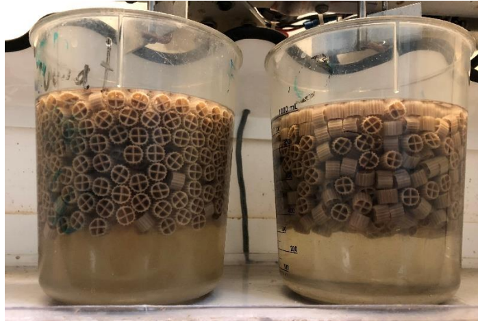
Figure 32: Difference in turbidity in the liquid phase after nitrite (left) and nitrate (right) batch experiments.
