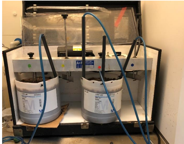
Figure 14: Experimental setup for the DO experiments by use of 3 L homemade containers. Low aeration was obtained by using one diffuser. High aeration was obtained using three diffusers.
