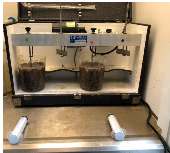
Figure 13: Experimental setup for anaerobic period of the batch experiments. Air pumps were aerating the batches through golf ball air stone diffusers in the aerobic period.
