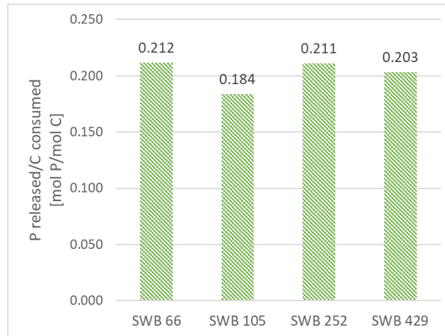
Figure 23: The rate of phosphate released per VFA consumed, given in mol P/mol C.
