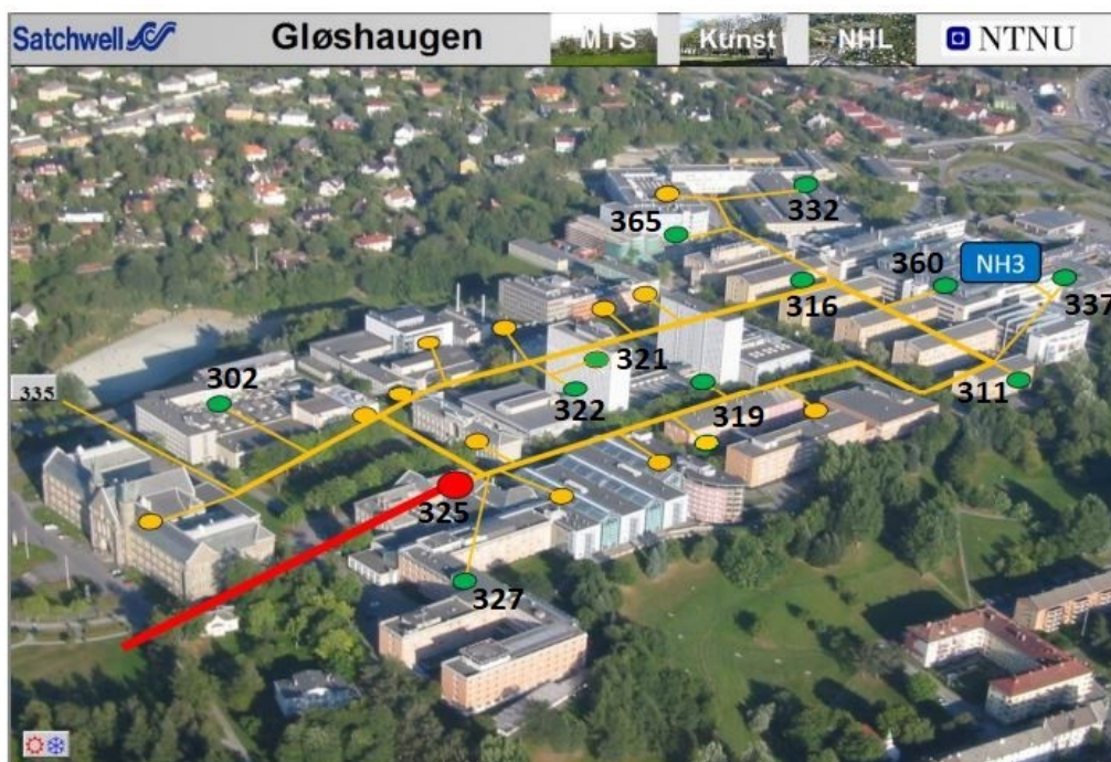
Figure 26. District heating ring on NTNU Gløshaugen (the yellow line) and the location of heat pumps (the green dots) ( Engan, Stene, & Høyem )
