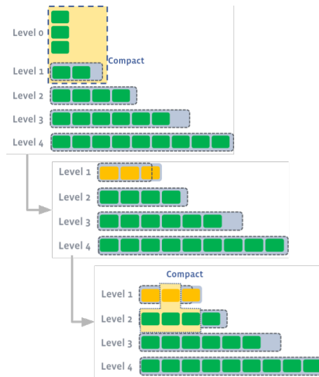
Figure 2.10: SS-tables from initial levels are compacted into the next [30].
