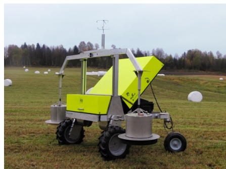
Fig. 1. A robot developed for autonomous N_2O measurements on cereal fields. The robots autonomy is currently under development where efficient attitude estimation is a focus.
