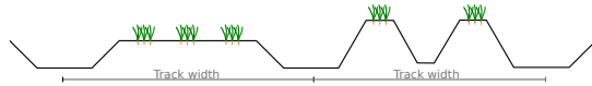
Figure 4: Carrots are typically triple-seeded in three rows on a lifted bed (left), or on two ridges between the tracks in the field (right). The track width is the distance across the row, measured from the center of the wheels of the machinery.
