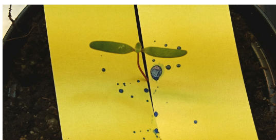
Figure 11: Chenopodium album L. after DoD application of liquid A3 with glyphosate. The liquid had very poor leaf retention properties, and satellite droplets were formed mid-air. No liquid is visible on the leaves, while the yellow liquid sensitive test strips highlight the droplets by turning blue. The droplets have either disintegrated in-air or bounced off the leaves.
