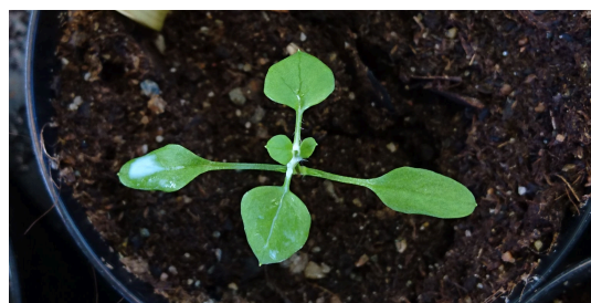
Figure 12: Stellaria media (L.) Vill. after DoD application of liquid A5 with iodosulfuron. The three applied droplets have spread and achieved good contact with the leaf.
