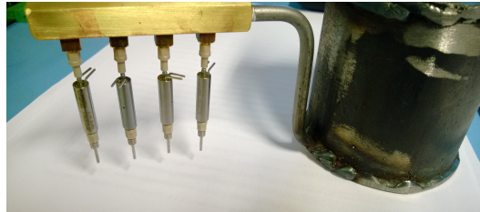
Fig. 7. Experimental setup with valves and pressurized liquid container, for early experiments with droplet formation, as shown in Figure 6 and 8.
