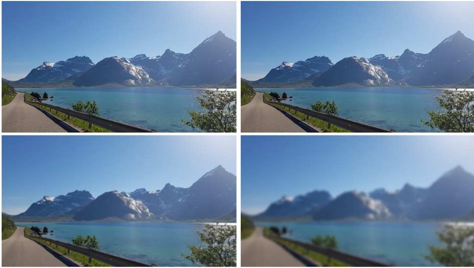
Figure 2.1: Gaussian smoothing applied to an image. Top left: original image. Top right: \sigma = 1 . Bottom left: \sigma = 5 . Bottom right: \sigma = 20 .
