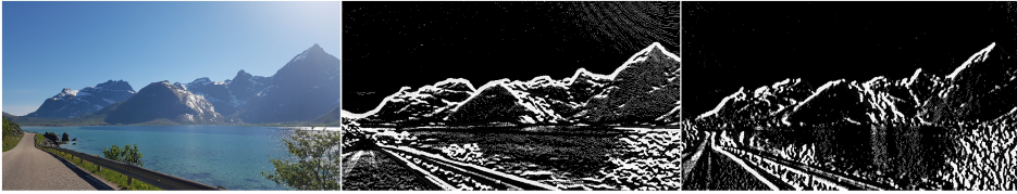
Figure 2.2: Sobel filter applied to an image. Left: original image I . Middle: K_y * G * I . Right: K_x * G * I .
