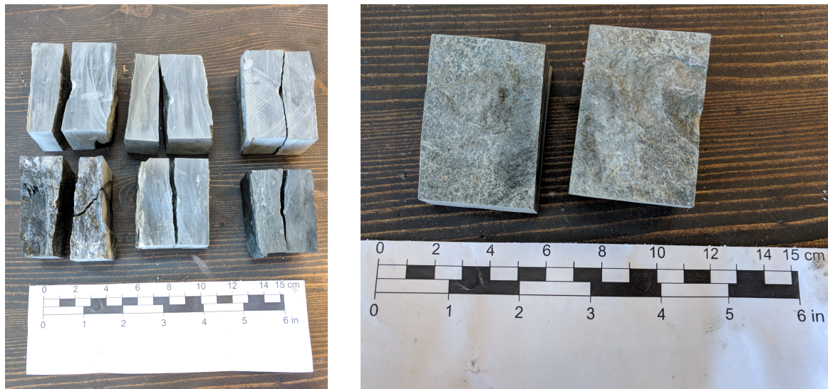
Figure 8.6: Fracture surfaces from testing parallel with the foliation plane
