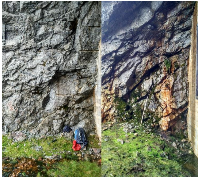
Figure 31 - Coarse-grained granite (left) and granitic gneiss (right) at the area of surge chamber. (Anna Helene Mong Urdal)
