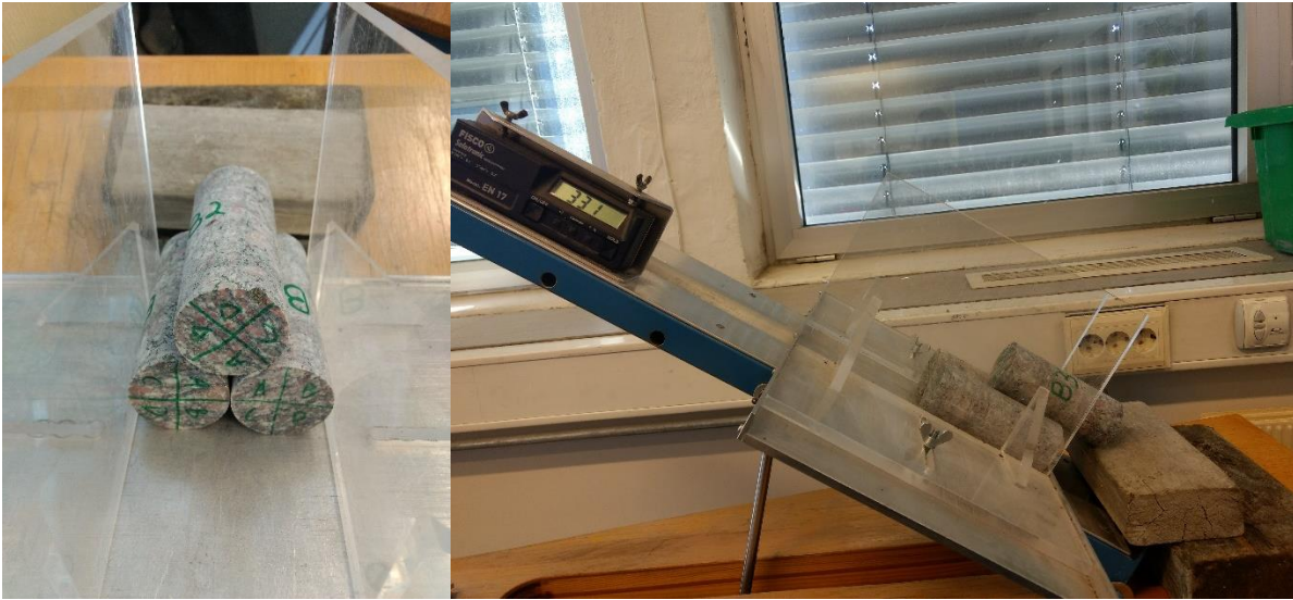
Figure 36 – (left) Three rock specimens from same rock sample, ready for tilt-testing of granite.
