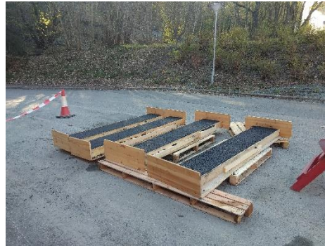
Figure 7 – Asphalt layers used in physical testing conducted by Peab Asphalt.
