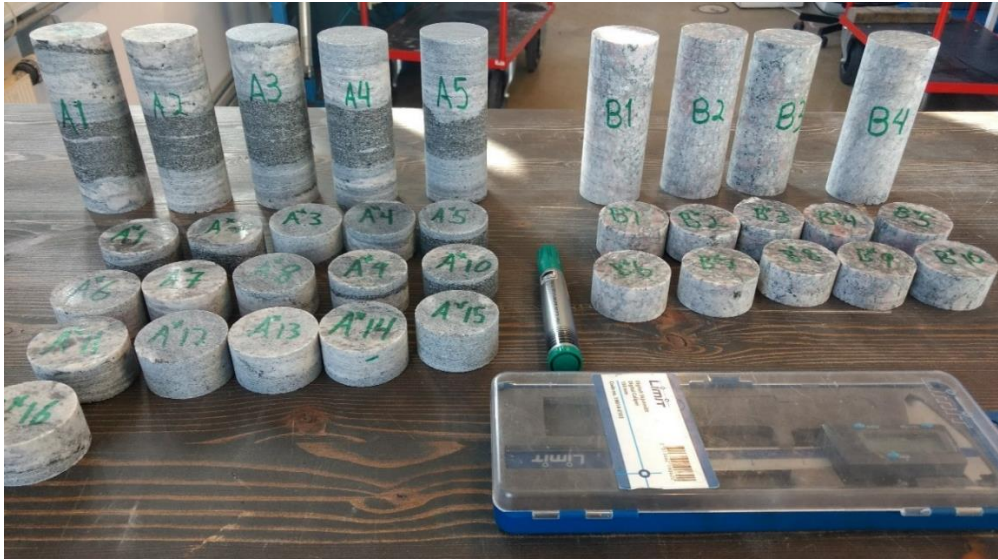
Figure 34 - Rock specimens used in laboratory testing. Group A represents the granitic gneiss and Group B represents granite. Both rock samples collected from Roskrepp area.
