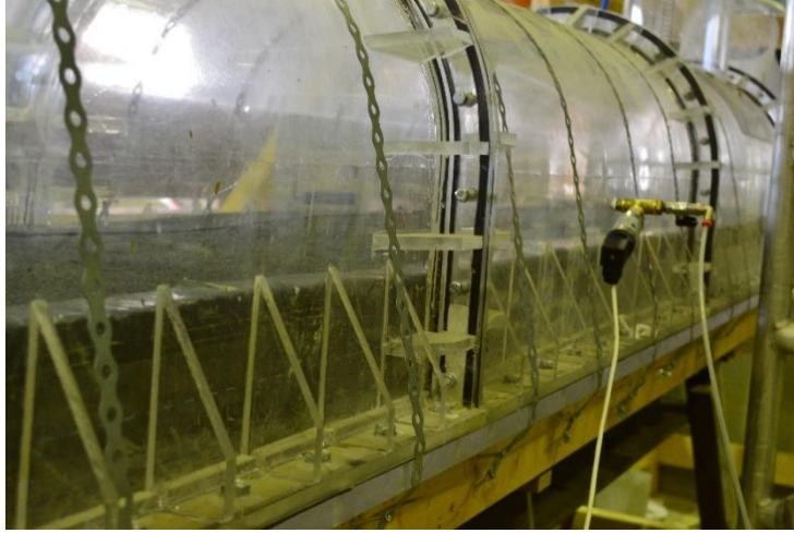
Figure 48 - Differential pressure sensor attached to the hydraulic model.
