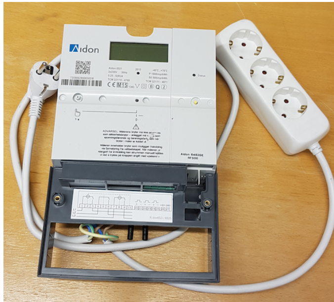
Figure 4.6: Slave meter with power strip installed.
