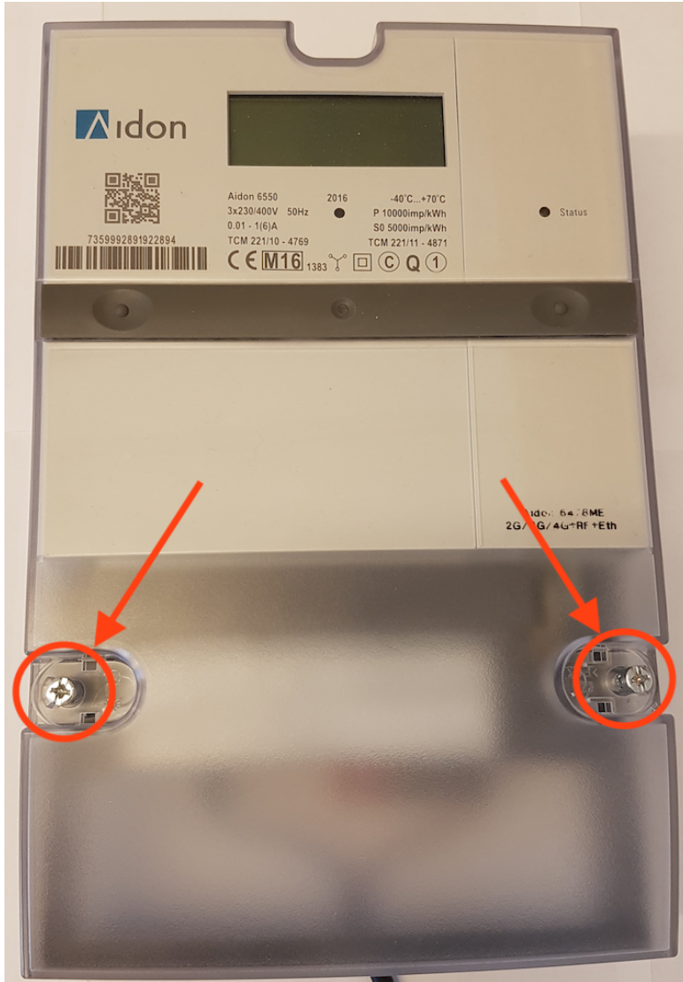
Figure 3.9: The indicated screws are used to attach the terminal sealing on the smart meter.
