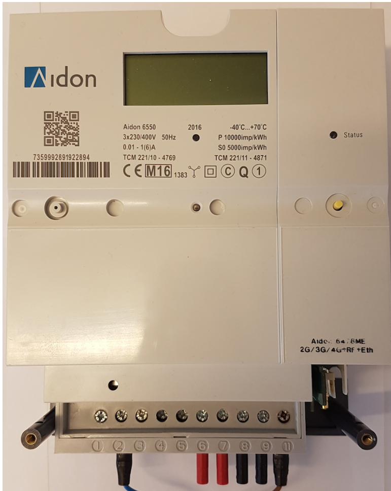
Figure 3.11: Smart meter with terminal sealing and interface protection removed.
