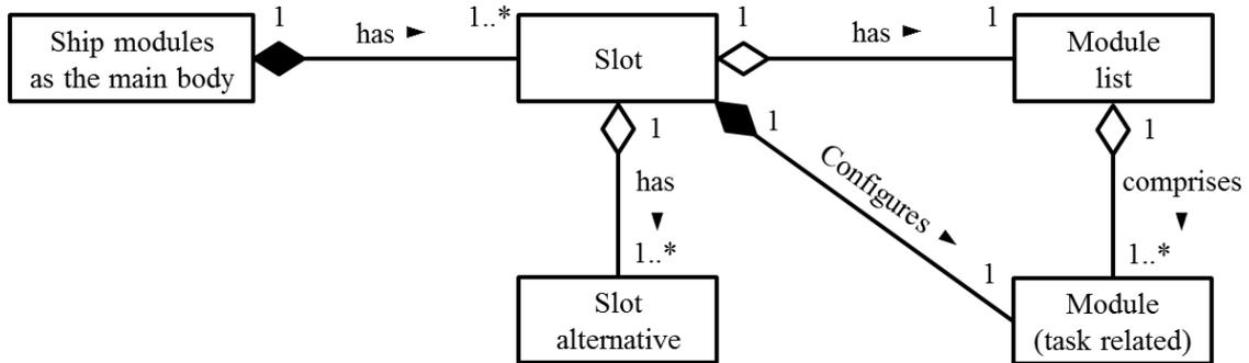
Figure 3. Description of ship modules, slots, and task-related modules using a class diagram in the unified modeling language.
