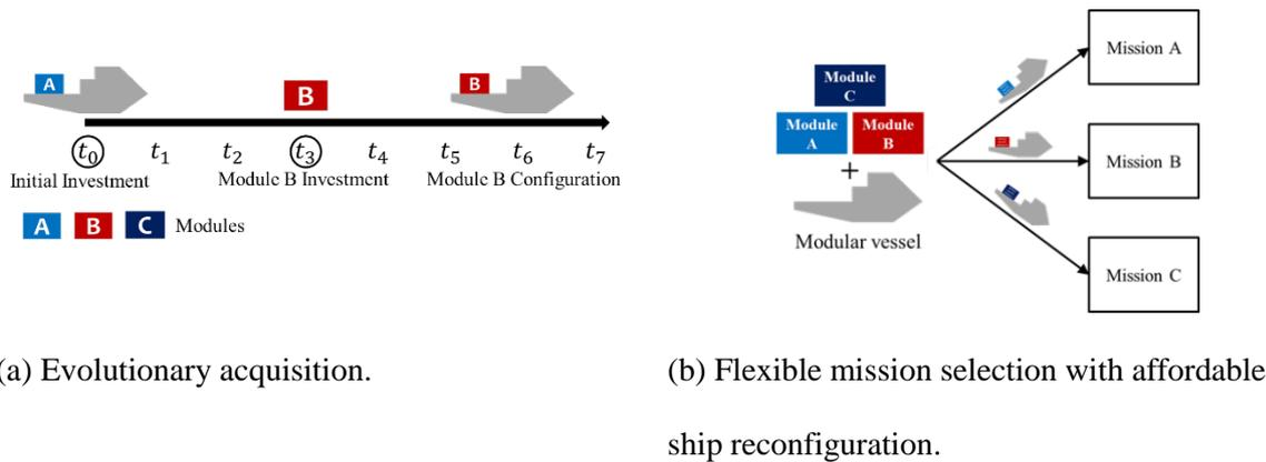
Figure 1. Operational flexibilities provided by modular adaptable ships.
