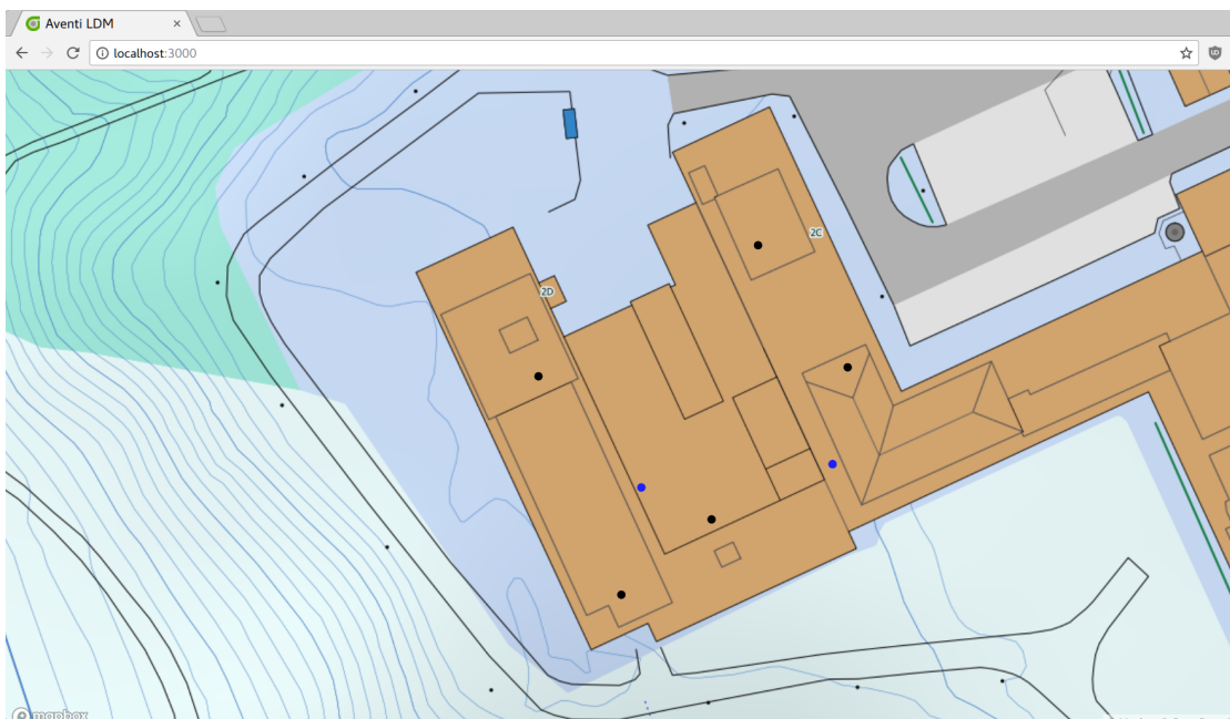
Figure 5.4: User frontend, showing the anchors as black dots and tags as blue dots on a map
