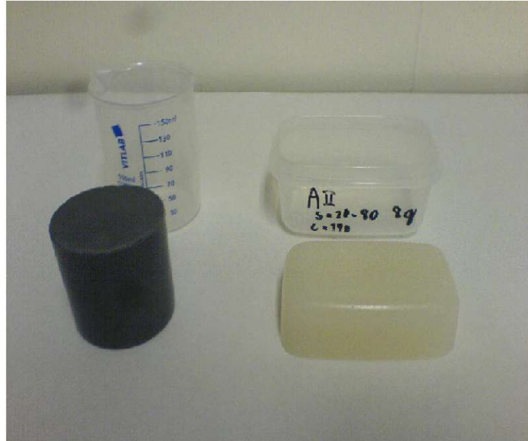
Figure 5.1: Phantoms made with silicium carbide (left) and sephadex (right).
