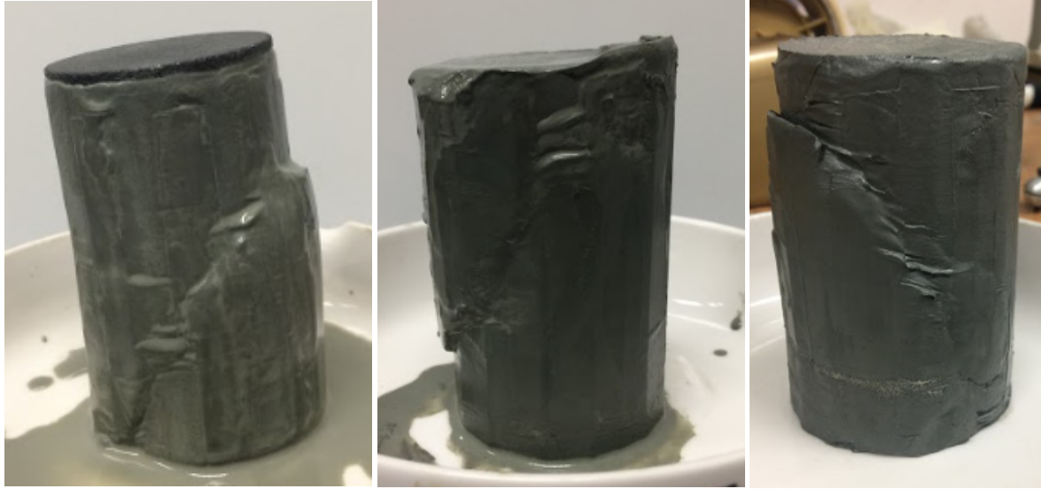
Figure 4.2: Failure patterns for three of the triaxial samples. All samples had a similar pattern.
