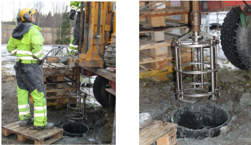
Figure 2.3: Block sampling at Flotten using a Sherbrooke block sampler.
