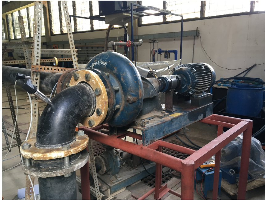
Figure 3.2: PAT test rig at UDSM: Water enters the PAT from the left in the picture, and exits in the foreground. To the right the shaft goes from the PAT to the generator, with a torque transducer in between.
