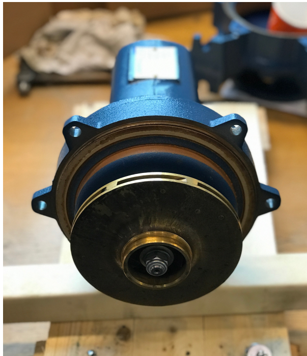
Figure 3.4: The pump impeller of Pedrollo FG 32/160B.
