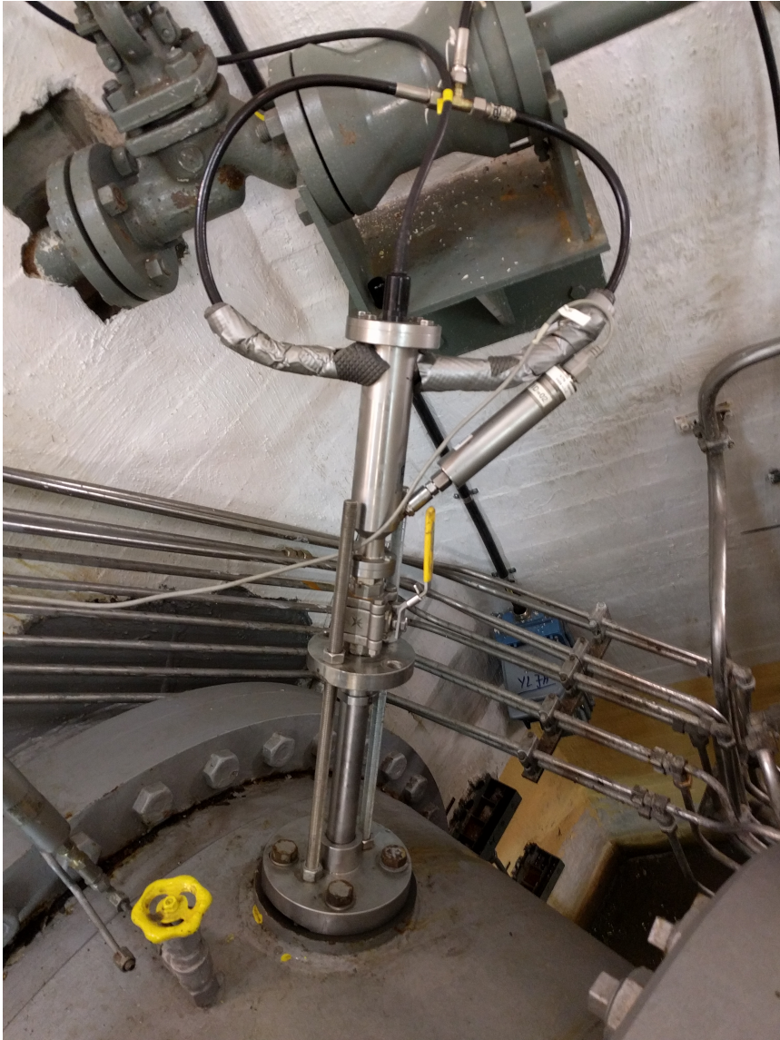
Figure 4.2: Probe on inlet, SBE38 black wire, Digiquartz white wire
