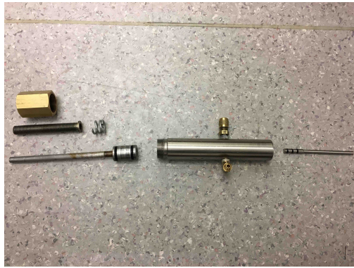
(a) The piston cylinder with a brass lid, threaded adjustable cylinder, big spring, big piston and small piston.
