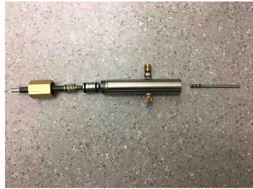
(b) All parts of the piston actuator aligned, ready to be assembled.
