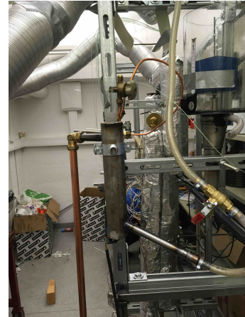
(c) The heating container mounted in the test rig. The oil supply tube can be seen on the right side, while the outlet of the heating container is to the left.
