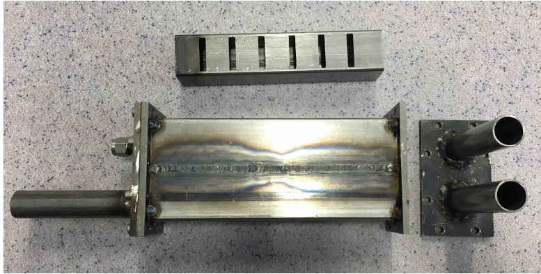
Figure 4.8: Sliding valve 1. The slider has six rectangular holes. On the left hand side is the lid with the piston rod penetration unit for the small piston and the outlet for the cold oil. On the right hand side is the inlet of oil and outlet for the hot oil. The profiles are welded together and the flanges are spot welded. Holes for the mounting bolts can be seen in the detached lid to the right.
