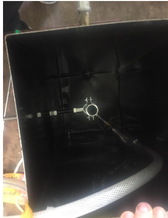
(b) Floating valve mounting with a hose clamp on the end of a threaded rod.
