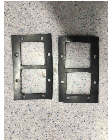
(c) Rubber gaskets to seal the flanges during tests with water.
