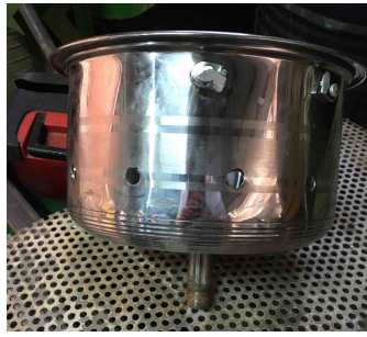
(b) Holes drilled in the medium cooking pot.
