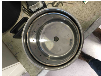
(a) Medium and large pot. Exit holes at the side walls of the medium pot and a hole in the centre for the inlet pipe.
