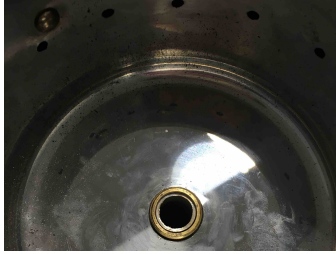
(a) The inlet pipe going through the large and medium pot, seen from inside the medium pot.
