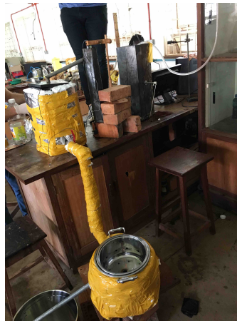
(b) The test setup at Makerere. Insulated parts are covered with yellow tape.
