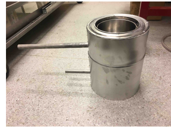
(c) The inlet pipe connected at the lower side and the outlet pipe connected at the upper side.
