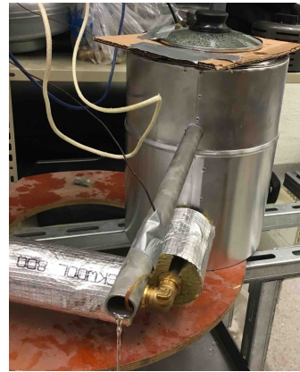
(b) A lid was covering the small pot containing water. Oil exited from the pipe coming out of the upper part of the cooking application.
