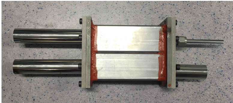
Figure 4.13: Sliding valve 3. Both the flanges and the profiles were glued using Loctite SI 5399.
