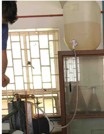
(a) The oil supply tank connected to the floating valve via a plastic hose.
