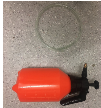
(b) The pressurised filler with a hose that connects it to the closing valve of the copper coil.
