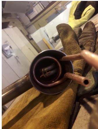
(a) Heating element with the copper coil fitted around, inside the heating container.
