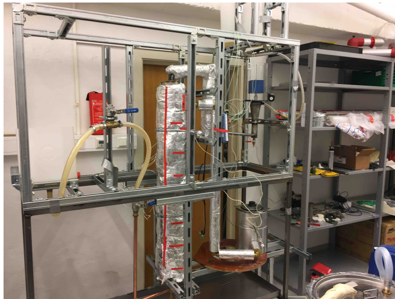
Figure C.4: The test rig made at NTNU. The cooking application is located low at the right hand side. The rock bed is located in the middle. The fill valve from the co-project is located above the cooking application.
