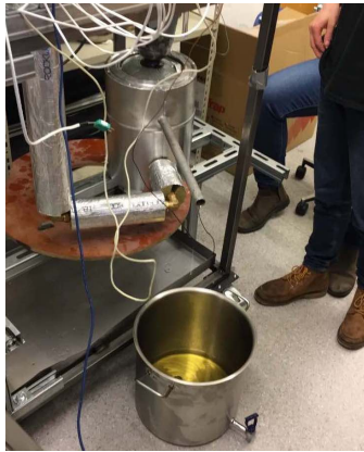
(a) The cooking application implemented in the full system, with the connecting pipes on the left coming down from the rock bed.
