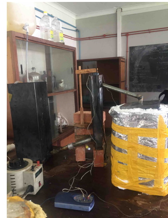
(c) The test setup at Makerere seen from behind. In front is the variac and pico logger for the thermocouples.
