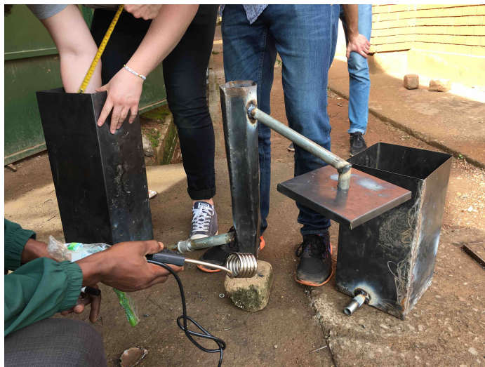
(a) The metal containers during production. From left to right: fill valve container, heating container and thermal heat storage. The heating element is held in front of the containers.
