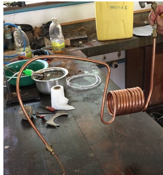
(a) The copper coil made for testing the movements of the pistons in the actuator.
