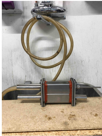
(a) Test setup for the sliding valves. The valves were filled with water using a plastic hose.
