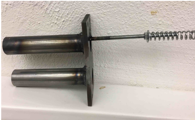
(a) Threaded rod with a nut to provide an adjustable foundation for the small spring. The rod was spot welded to the inlet pipe.
