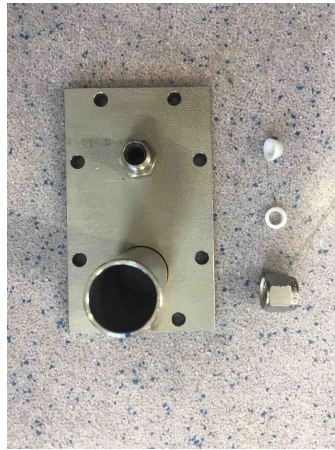
(b) Lid with the piston rod penetration unit made out of a Swagelok fitting. The PTFE gaskets and tightening bolt are placed on the right hand side.
