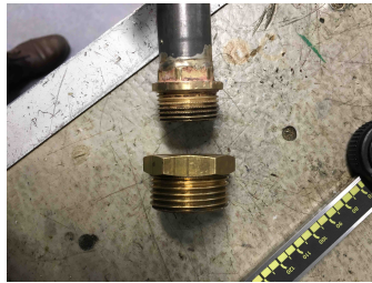
(b) The soldered pipe with its nut, before cutting, for attaching the medium and large pot together.
