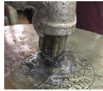
(c) Clumpy welding on the cooking application with silicon sealant.
