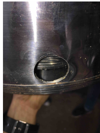
(e) Gap between the medium and large cooking pot due to clumpy welding.
