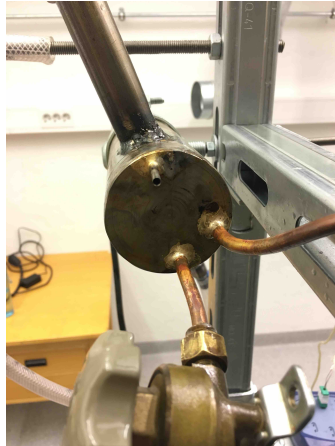
(b) The top lid of the heating container with the copper coil and thermocouple pipe soldered to seal the penetration.
