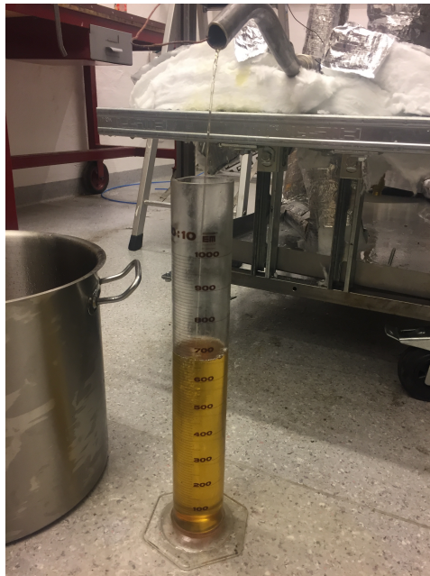
Figure 3.9: Measurement of the mass flow rate
