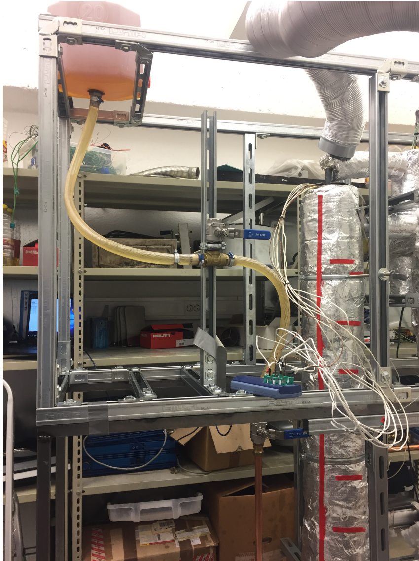
Figure 3.45: Heat storage ready for reversal
