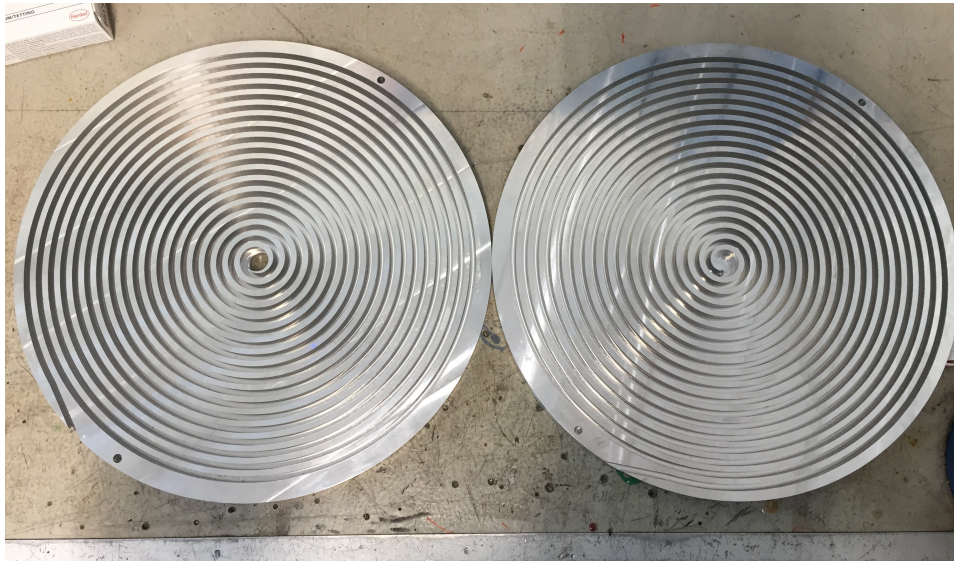
Figure 3.43: CNC milled griddle parts
