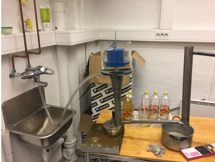
Figure 3.27: Fill valve test with water
