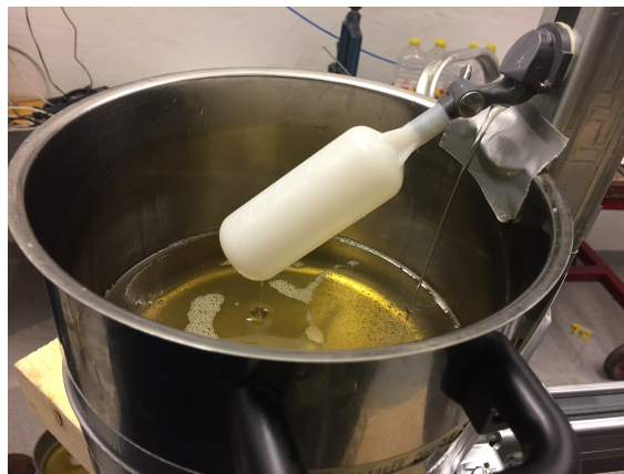
Figure 3.29: Aquarium fill valve test
