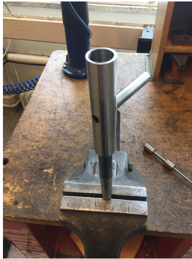
Figure 3.21: Reaming the "T" manually
