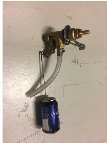
Figure 3.12: Piston Fill Valve
