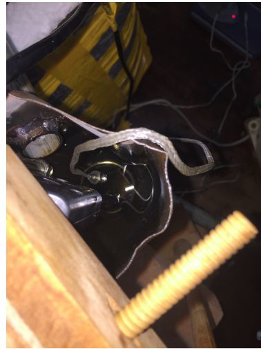
Figure 4.17: Heating element and thermocouples
