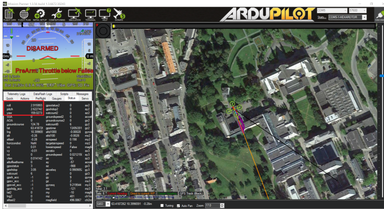
Figure 5.1: The Mission Planner interface. The “Status” page shown on the right allows quick and easy access to some of the most mission critical data. The UAV’s orientation, roll, pitch and yaw, are highlighted by the red bounding box.
