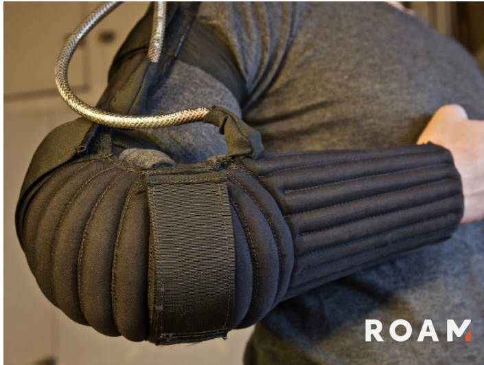
Figur 8.4: Roam Robotics sin fluid-drevne aktuator [13].
