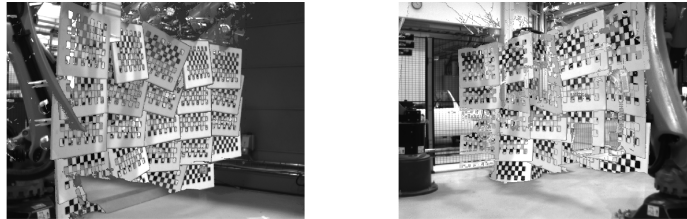
Figure 7.4.: A composite of the calibration images taken with the left and right camera respectively.
