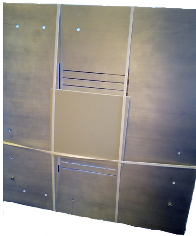
Figure 3.35: Superstrate held in place by rubber bands
