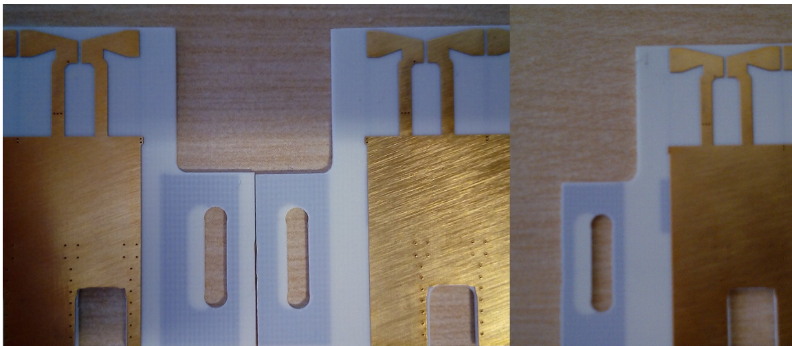
Figure 3.31: Picture of production error in layer 3 of the PCBs
