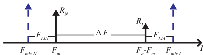
Fig. 3. Sketch of parts of the detector signal spectrum. The black solid arrows indicate the R_I and R_N signals, and the stippled arrows the local oscillator signals defined in Eqs. (6) and (7).
