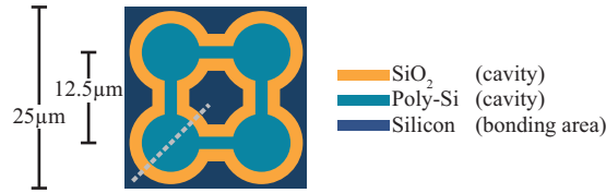
Fig. 6. The etched out cavities in a cell consists of four circular CMUTs with connection bridges. Note that only the darkest areas are in contact with the top plate. Figure 5 illustrates the cross section along the dashed line.
