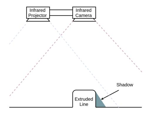
Figure 5.1: Working Principle of Structured Light Camera.
