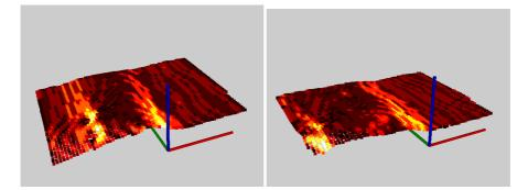
Figure 4.15: Overfilled extrusion at 120mm, line 2 to the left and line 4 to the right.
