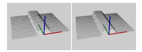
Figure A.5: Straight line with noisy data. Unfiltered to the left, Smoothed out by gaussian kernel to the right.
