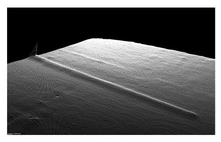
Figure 4.3: View of one extruded line with the the extruder tool tip set to 3mm above the table. Extruding from right to left. Point cloud captured at end of line extrusion.
