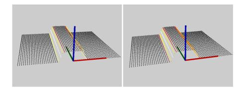
Figure 3.6: Calculated gradient with Sobel operator. Unfiltered to the left, Smoothed out by Gaussian kernel to the right.
