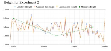
Figure B.3: Experiment 2 height plot using the Sobel gradient.
