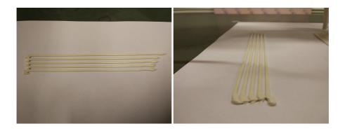
Figure 4.8: Underfilled extrusion.
