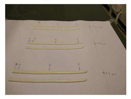
Figure 4.2: View of the three pairs of different single layer tests, with 3mm at the top and 5mm at the bottom.
