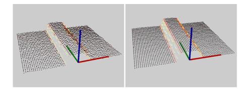
Figure A.6: Straight line with noisy data. Calculated gradient with Sobel operator. Unfiltered to the left, Smoothed out by gaussian kernel to the right.
