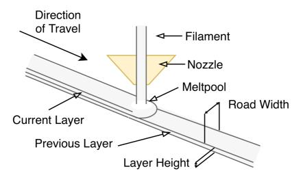
Figure 2.1: General principle of additive manufacturing using filament
