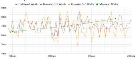
Figure B.10: Experiment 5 width plot using the Sobel gradient.
