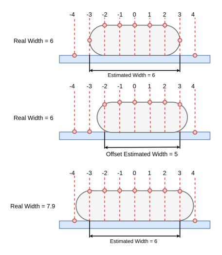
Figure 3.7: Quantization errors for a scanner with resolution of 1.
