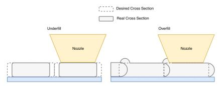
Figure 2.2: Under- and overfill errors along parallel paths
