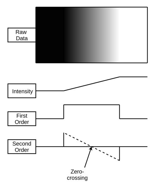
Figure 2.5: General connection between intensity, first order and second order derivatives
