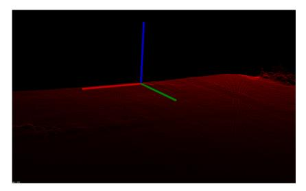
Figure 3.4: Transformed point cloud with the surface of the work table as zero in z-direction. We see that the surface of the point cloud fits the displayed coordinate frame.
