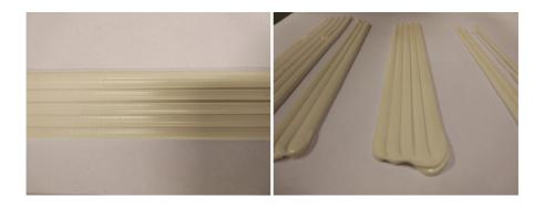
Figure 4.7: Normally filled extrusion.
