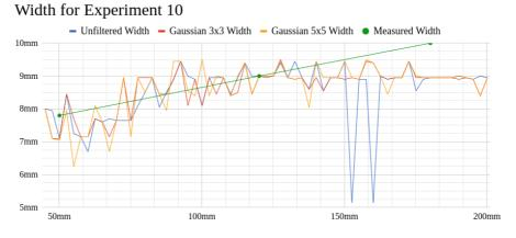
Figure B.20: Experiment 10 width plot using the Sobel gradient.
