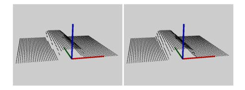
Figure A.1: Incremental offset as a point cloud. Unfiltered to the left, Smoothed out by gaussian kernel to the right.
