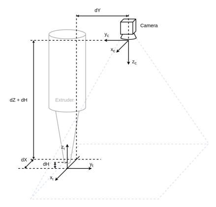
Figure 3.1: Relation between coordinate frame of the camera and the extruders coordinate frame
