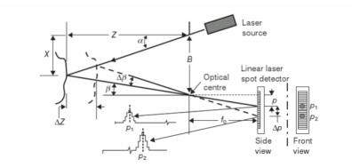
Figure 2.4: Basic principle of distance measurement using triangulation, from [1]
