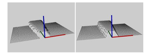
Figure A.3: Incremental width as a point cloud. Unfiltered to the left, Smoothed out by gaussian kernel to the right.
