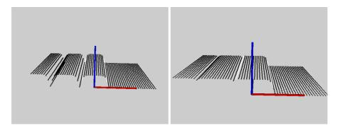
Figure 5.2: Wide underfill valley to the left, narrow underfill to the right.
