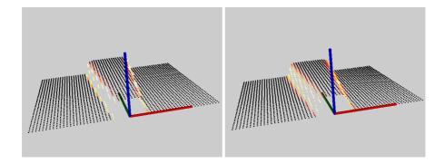
Figure A.4: Calculated gradient with Sobel operator. Unfiltered to the left, Smoothed out by gaussian kernel to the right.
