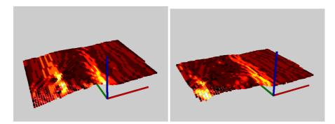
Figure 4.13: Underfilled extrusion at 120mm, line 2 to the left and line 4 to the right.
