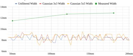
Figure B.26: Experiment 13 width plot using the Sobel gradient.
