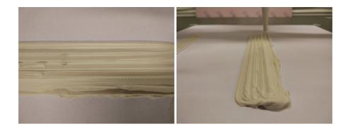
Figure 4.9: Overfilled extrusion.
