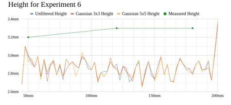
Figure B.11: Experiment 6 height plot using the Sobel gradient.
