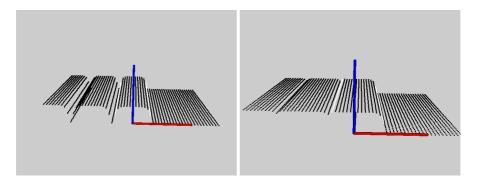
Figure 5.5: Wide underfill valley to the left, narrow underfill to the right.
