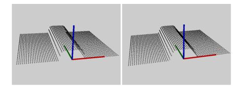
Figure 3.5: Straight line as a point cloud. Unfiltered to the left, Smoothed out by Gaussian kernel to the right. There is only a slight visible smoothing of the edges closest to the "floor".
