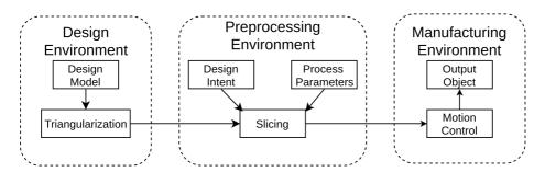
Figure 2.3: General Software-toolchain for Additive Manufacturing process
