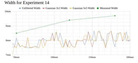
Figure B.28: Experiment 14 width plot using the Sobel gradient.
