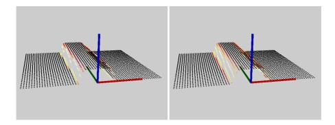
Figure A.2: Calculated gradient with Sobel operator. Unfiltered to the left, Smoothed out by gaussian kernel to the right.
