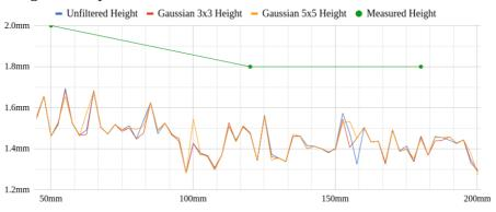
Figure B.13: Experiment 7 height plot using the Sobel gradient.
