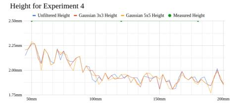
Figure B.7: Experiment 4 height plot using the Sobel gradient.
