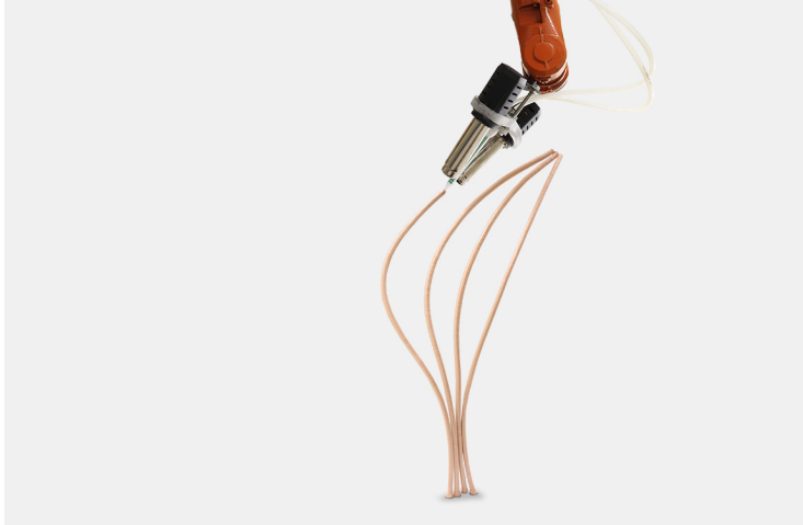
Figure 2.3: The Mataerial project enables AM along double curved lines in mid-air. Image courtesy of Mataerial (2018)
