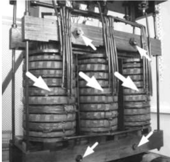
Figure 26. Transformer presenting a third degree mechanical defect of the active part (Borucki, 2012)
