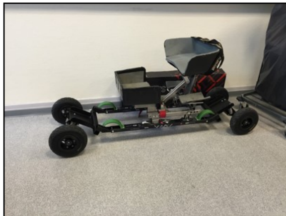
Figure 1.3: Prototype Alpha: The first off-road cross-country sit-ski prototype. Source: Steering system for cross-country sit-skis [6]
