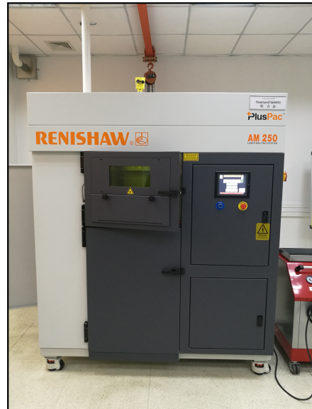
Figure 3.9: Metal 3D-printing, 250x250x30 mm
