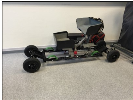
Figure 1.2: The first off-road cross-country sit-ski prototype.
