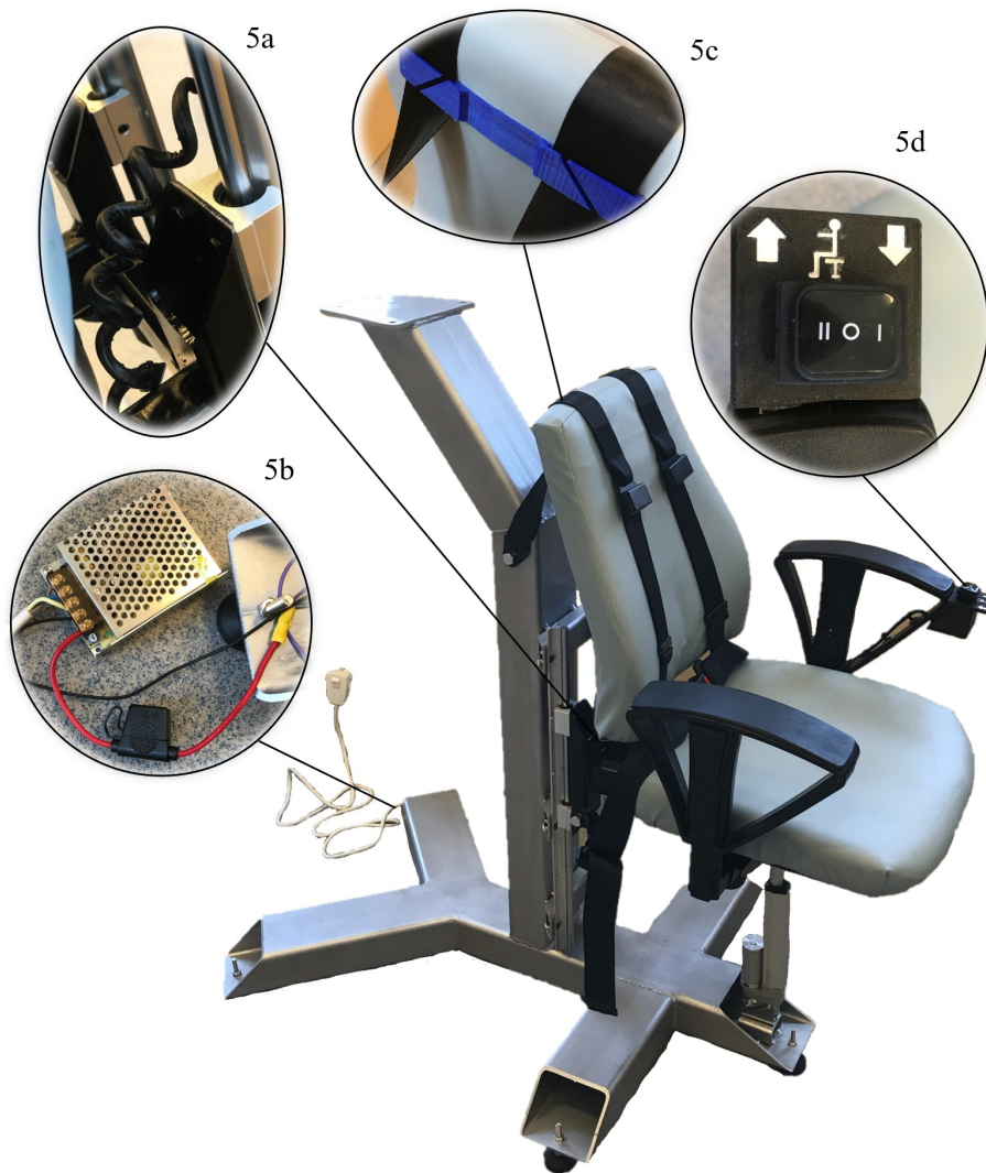
Figure 5.53: Proof of concept prototype with pig tailed wire (5a), power supply (5b), seat belt clip (5c), and DPDT switch (5d).
