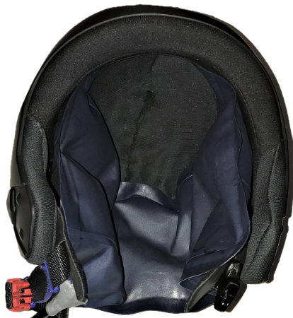
Figure 5.27: Head mount with inflatable pillow
