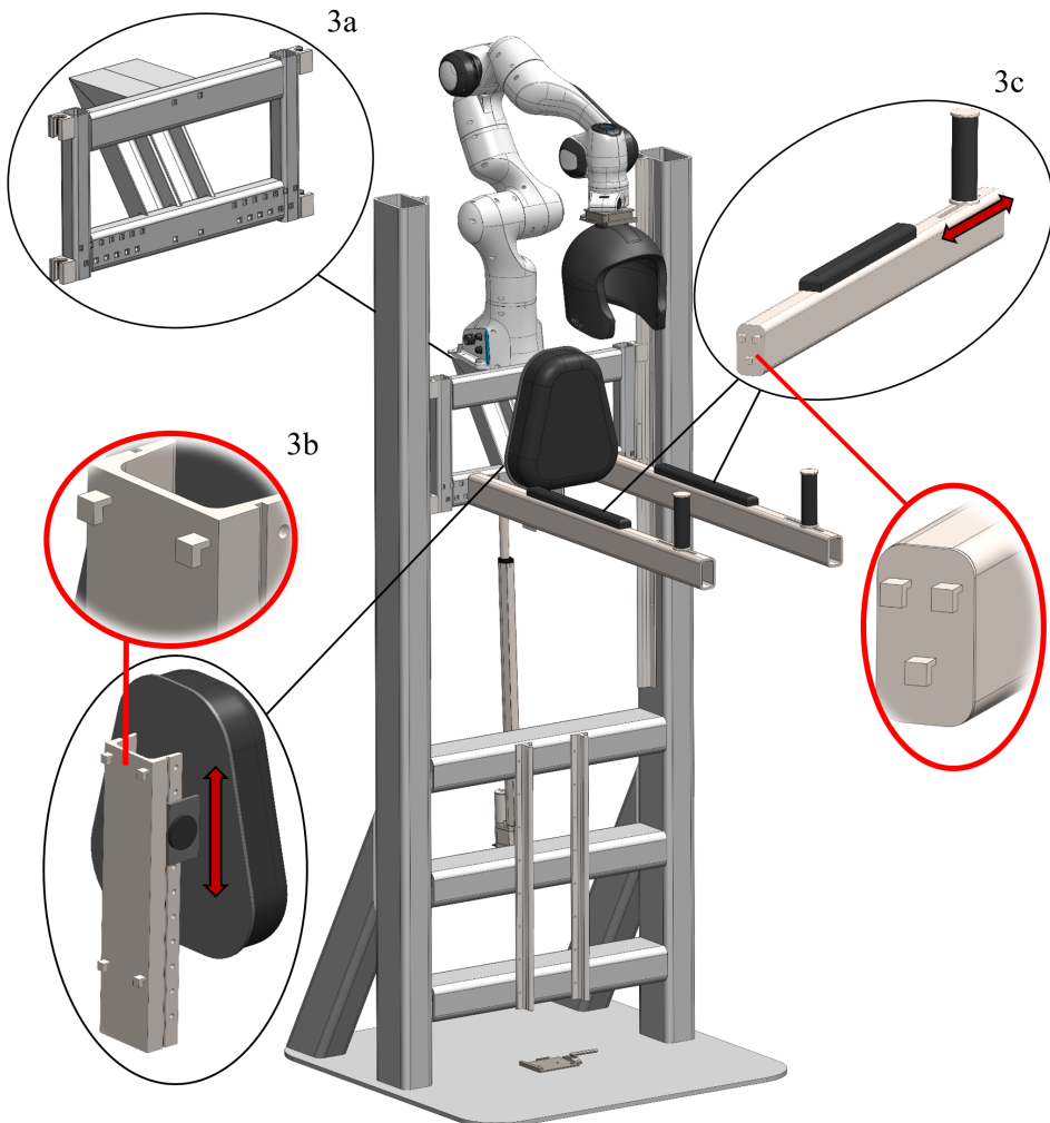
Figure 5.46: Assembly of Hybrid design, standing version, with custom made base fixture (3a), adjustable backrest (3b) and armrests (3c).
