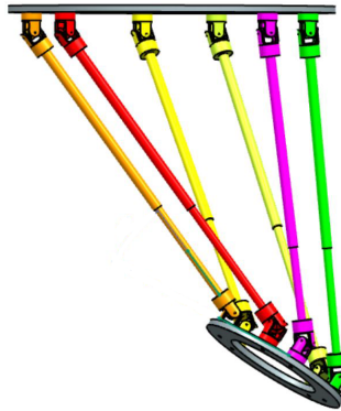
Figure 4.1: Stewart platform from Slåttsveen and Tolo thesis [41].
