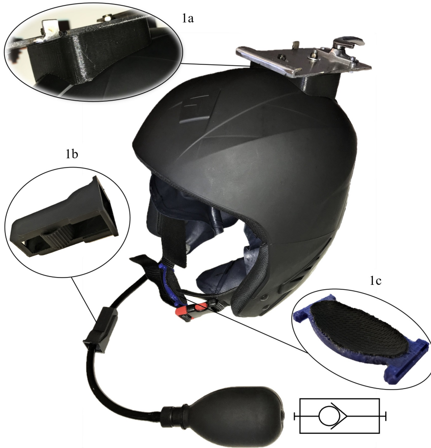
Figure 5.25: Head mount concept consisting of: mounting shim (1a), stop valve (1b), chin strap (1c), bulb pump and customized inflatable.
