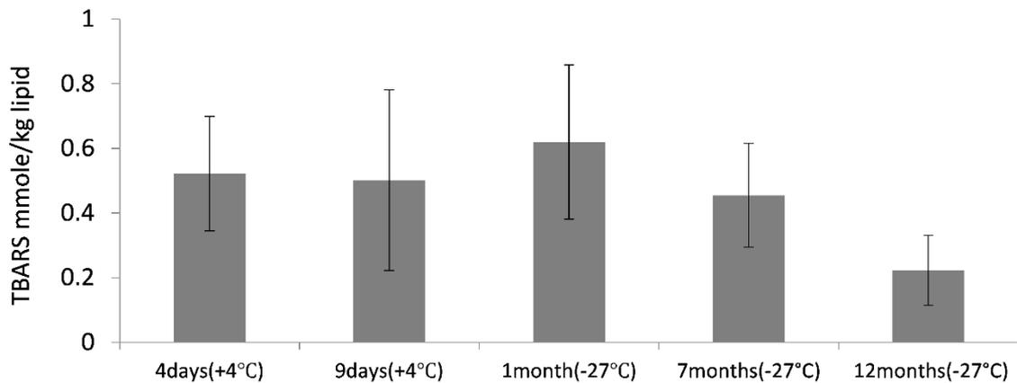
Figure 2 TBARS values in total lipids extracted from whole mackerel fillets with skin (mmole/kg lipid) stored at +4°C and -27°C. The values are given as an average of at least three samplings, with standard deviations.
