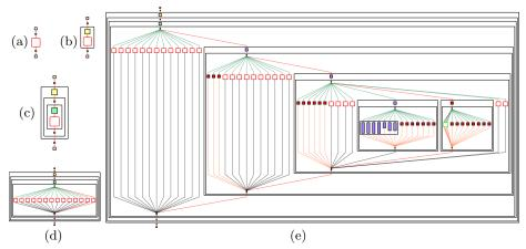
Fig. 4. Navigating the aggregated grain graph of NQueens program from BOTS for high-parallelism input (n=14, cutoff=4). The graph has 21492 grains and 3073 group nodes. Grains with low parallel benefit are highlighted as problems. (a-d) Drilling down to sibling groups at a depth of 3 from the root group. (a) Root group. (b) At depth 1. (c) At depth 2. (d) At depth 3. (e) Drilling down along the critical path to sibling groups at the lowest depth.
