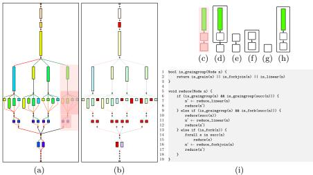
Fig. 2. Grain graph of the task-based Sort program from BOTS for small input (n=512, cutoffs={256,64,16}). (a) Structural view (b) Problem view highlighting low parallel benefit in red (c) After two fork-join pattern reductions of the highlighted subgraph (d-g) Linear pattern reductions leading to a single group node (h) After normalization (i) Reduction pseudocode
