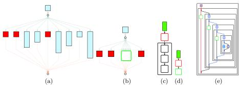
**Fig. 3.** Separation of problematic from non-problematic nodes. (a-b) Fork-join node separation. (c-d) Linear node separation. (e) Local (blue) and global (red) critical paths
