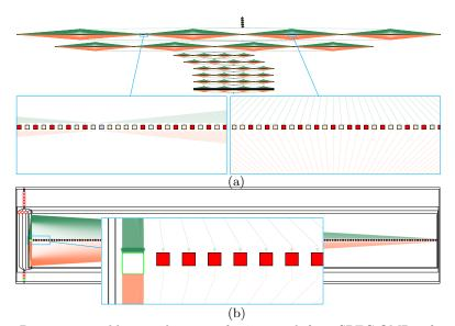
Fig. 5. Diagnosing problems with grains of 367.imagick from SPEC-OMP12 for input -shear 31 -resize 1280x960 -negate -edge 14 -implode 1.2 -flop -convolve 1,2,1,4,3,4,1,2,1 -edge 100 ref/input/input1.tga. (a) Sweeping across the entire unaggregated graph with 3801 grains to spot problems. (b) Aggregated grain graph enables programmers to diagnose problematic grains group-wise. Non-problematic grains are separated to promote focus (inset).
