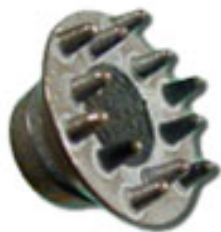
Figure 3.4: Picture of a dry electrode from Florida Research [53]. There are in total eight of these attached to the headset.
