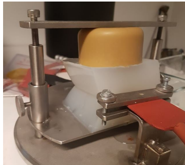
Figure 3.5: Experimental setup used for determining thermal conductivity in agar-gel
