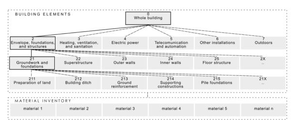
**Figure 2.** The hierarchical structure of the building elements according to NS 3451, and the material inventory. The elements with bold outlines are expanded to show their sub-elements. Each building element has its level ID above its name. The inventory items are connected to specified building elements.
