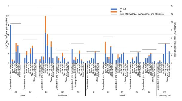
**Figure 3.** The embodied emissions in  $kgCO_2e./m^2year$  from material production (A1–A3) and replacements (B4) for 11 buildings from four different typologies. The building elements in the category "Envelope, foundation, and structure" are shown for each building (left axis) together with the total for this building element (right axis).
