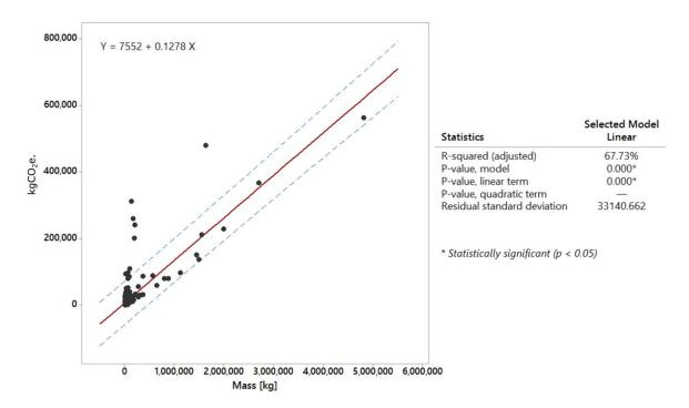
**Figure 5.** The weight of all inventory items plotted against emissions from material production (A1–A3) in kgCO<sub>2</sub>e., together with a regression model of the correlation. One outlier which is related to a special case of ground reinforcement was removed.
