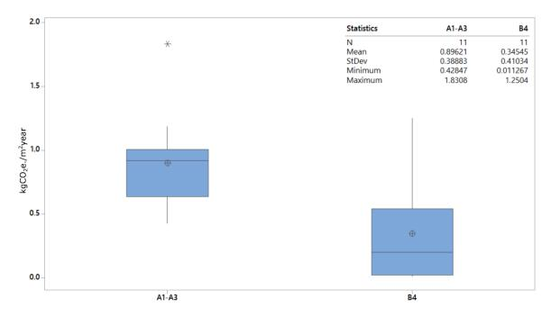
**Figure 4.** The distribution of embodied emissions per floor area and a lifetime of 60 years for the outer walls of the 11 buildings (kgCO<sub>2</sub>e./ $m^2$ year).
