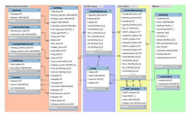
Figure A1. The Entity-Relationship Diagram (ERD) of the database used for storing the data.
