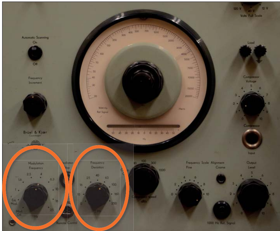
Figure 3.5: Close up on the modulation controls on a Brüel & Kjær BFO 1022, a model similar to the BFO Nordheim was using. Photo: Ola Nordal.
