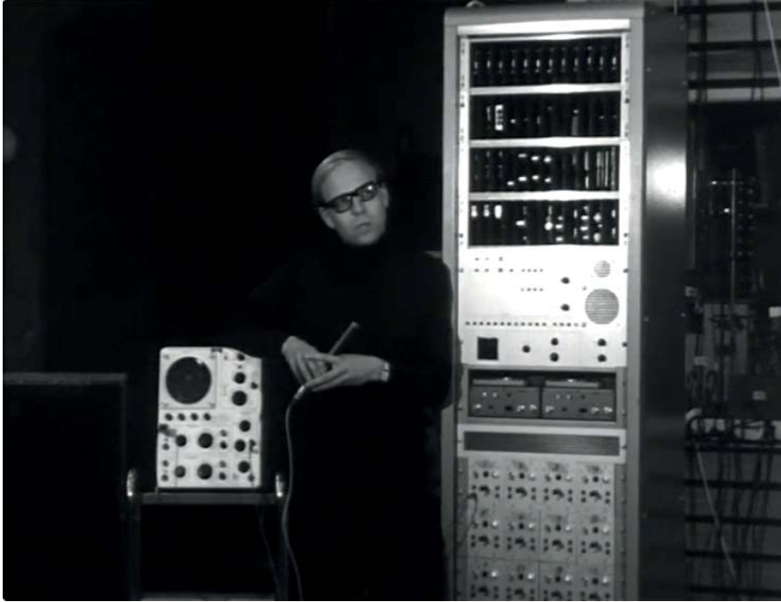
Figure 5.13: Nordheim in front of his Music Machine. Eva Brustad. "Lydskulptur", NRK TV, October 25 th 1968. The amplifiers can be seen in the bottom of the rack. Tape machines in the middle of the rack.
