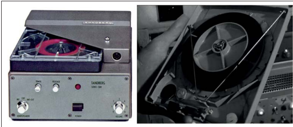
Figure 5.14: Left: Tandberg 1324 'endless' tape loop machine, similar to the one Nordheim used. Right: "Endless" tape loop cassette used in Ode to Light 391
