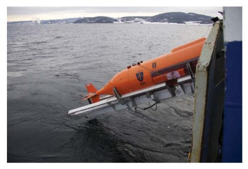
Figure 2.4: Hugin AUV being deployed from RV Gunnerus
