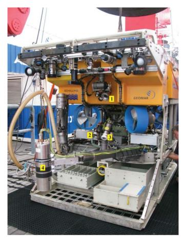
Figure 3.2: The camera setup of ROV Kiel 6000: Upper Pan & Tilt Unit with SD Camera (1), AQUOREA strobe and halogen light. Lower Pan & Tilt Unit with SD Camera (2), HD Camera (3) and halogen light. The Underwater Hyperspectral Imager (4) can be seen mounted on the extended manipulator arm.
