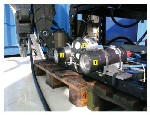
Figure 3.1: The NTNU stereo camera (1) rig with a horizontal DVL (2) mounted on ROV  $30\mathrm{K}$
