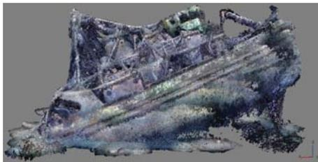
Fig. 6. Dense point cloud model seen from starboard
