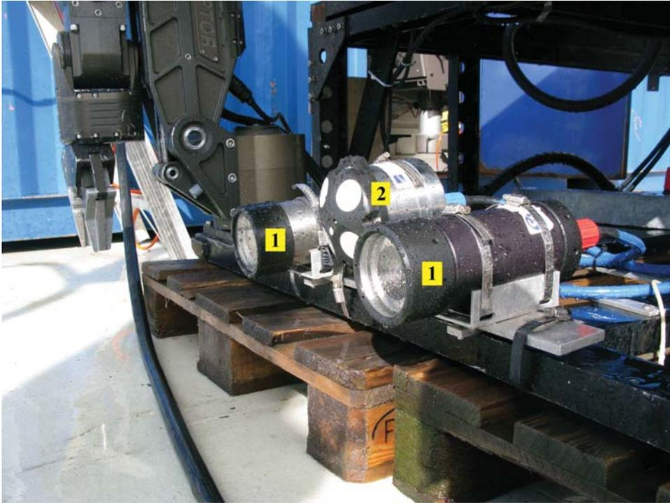
Figure 3.1: The NTNU stereo camera (1) rig with a horizontal DVL (2) mounted on ROV 30K
