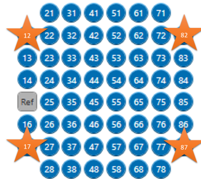
(e) Investigated electrodes (marked in stars) are physically located in each corner of the MEA.
