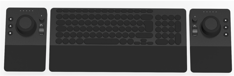
Figure 3.6: Intuitive Input Device (IID) from Inventas AS. Note that the device consists of the two platforms on either side of the keyboard, as well as an control box not shown in the figure. Image courtesy: Inventas AS
