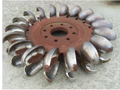
Figure 1.2: A Pelton turbine wheel, the split buckets are easily visible. By Zedh.
