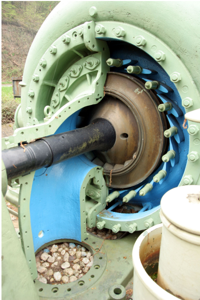
Figure 1.3: Cross section of a Francis turbine. The guide vanes are seen in almost closed position. By Armin Kübelbeck. a
