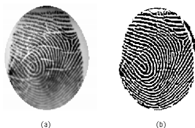
Figure 6.12: An experimental result of fingerprint enhancement method proposed by Luo et al. [159]. (a) represents the original fingerprint, and (b) represents the enhanced image.
